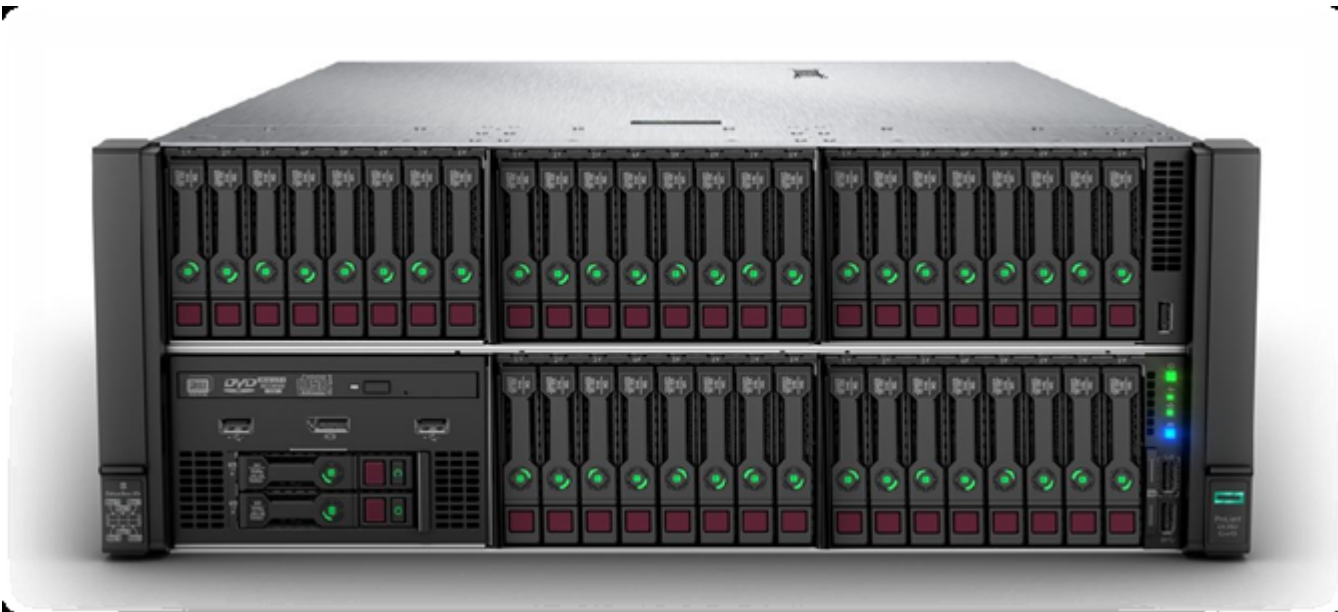
40 SFF hot-plug drive model and 2 NVMe SSDs with Universal Media Bay
